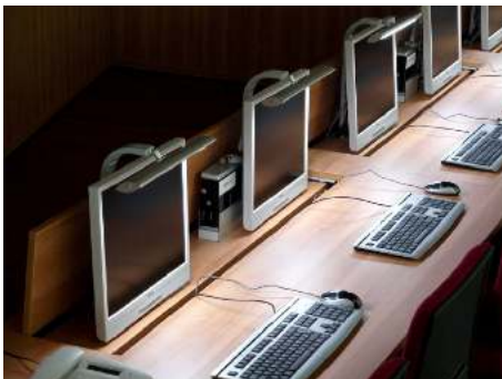
The Thin Clients come from inside the desk and can always be used immediately. If no technology is required, they are lowered back in.
